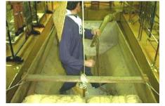
Robeso; the navel of Ro (pivot) and Ro-nawa( rope) are offsetted from the center of the boat.
